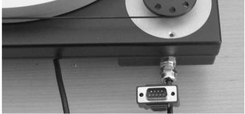
position and the speed selector is on 33 rpm. Then plug in the 3-pin connector from the external AC/AC adaptor to the plug on the back of the PS800. Then connect the main
