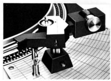
By the smooth movement of rackand-pinion, the balance-weight can be easily adjusted. After you get the balance, pull the balancing knob outward, and the scale will return to zero instantly. Now you can add any amount of tracking force you desire by directly reading the scale on the knob, a special device developed for convenient operation. For those who prefer to use more than one cartridge, this is it.
