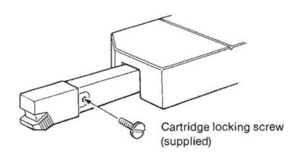
Plug the cartridge (optional) into the tonearm and tighten the cartridge locking screw firmly. The screw cannot be installed from the opposite direction.
