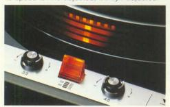
When you desire to change the fine adjustment, use the two independent fine speed controls, one each for the 45 and 33½ rpm speeds. Control latitude is ±2.5% for each. The precision stroboscopic pattern on the platter edge lets you visually check speed accuracy. It is illuminated by a bright neon strobe lamp for easy reading.
