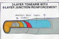
a tapered six-layer structure is used. This careful design is largely responsible for the accuracy and clarity of reproduction across the audible range, particularly at low-level low frequencies that are most difficult to reproduce authentically.
