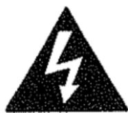
The lightning flash with arrowhead symbol within an equilateral triangle is intended to alert the user of the presence of uninsulated "dangerous voltage" within the product's enclosure that may be of sufficient magnitude to constitute a risk of electric shock to persons.
