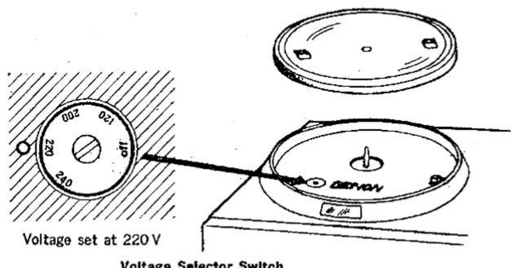
Fig.4 Voltage Selector Switch
