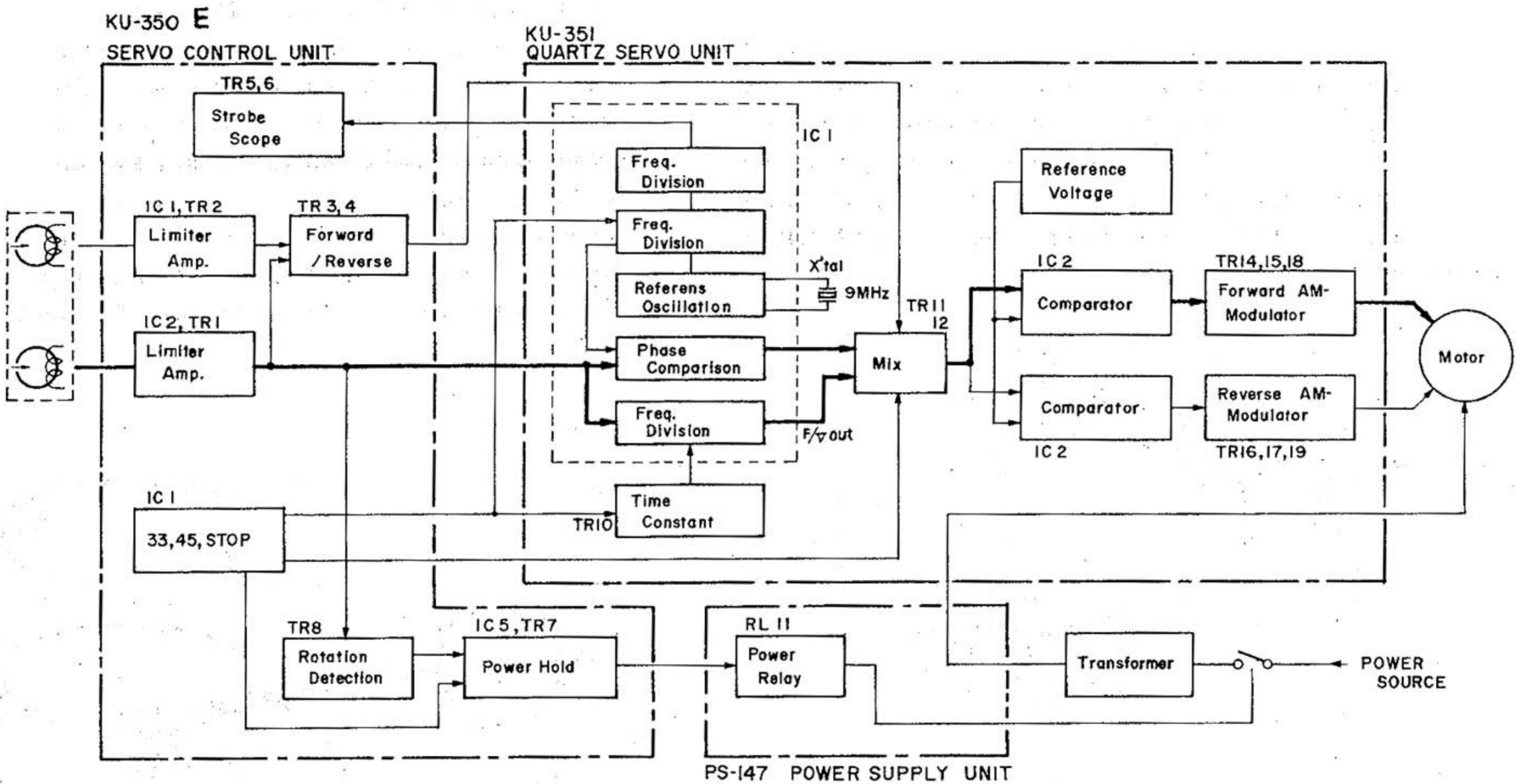
Fig. 1 Block Diagram of DP-75
