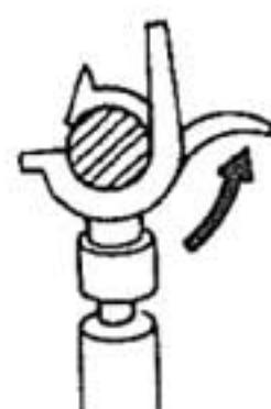
Return the tonearm to the arm rest and hold it in place with the clamp.
