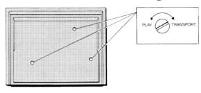
Before using the record player you must loosen the three transport screws underneath it. Place the record player on a table, with its front protruding over the edge of the table. Hold the record player firmly and turn it carefully until you have located and loosened each screw. The screws cannot be removed from the holes but should be turned several times using a screw-driver or a coin.
