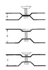
Turn the transport screws counter-clockwise towards stop.
