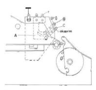
Adjust tags B and C so that on the pickup being raised contact will first be made between A and B (short-circuiting the channels together) and thereafter between A and C (Short-circuiting the signal).
