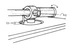
Turn the stylus-force adjustment screw to 0.
