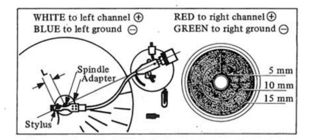
Your AP-005 is supplied with a 45 r.p.m. Adapter for use when playing 45 r.p.m. speed discs with a large center hole. Place the adapter on the turntable spindle.
