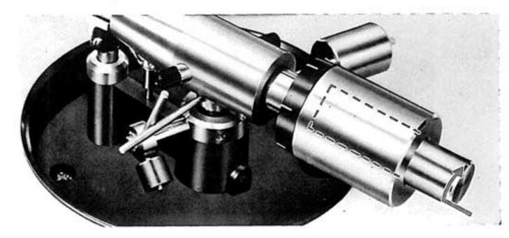
When using an exceptionally heavy optional cartridge (from 8 to 12.5 grams), to obtain perfect tone arm balance and stylus pressure, it may also be necessary to use the standard accessory Sub Weight. In this case, screw the Sub Weight into the opening at rear of the Main Weight and follow the above Tone Arm and Stylus Pressure Adjustment as well as Lateral Balance Adjustment procedures. Tighten to position at which tone arm balance is attained.
