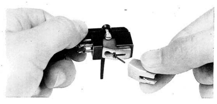
If the stylus is worn or the disc damaged, distorted or uneven sound will prevail during playback. If the stylus appears to be worn, replace with an ATS-11 or a 4 channel stereo stylus for CD-4 use.
