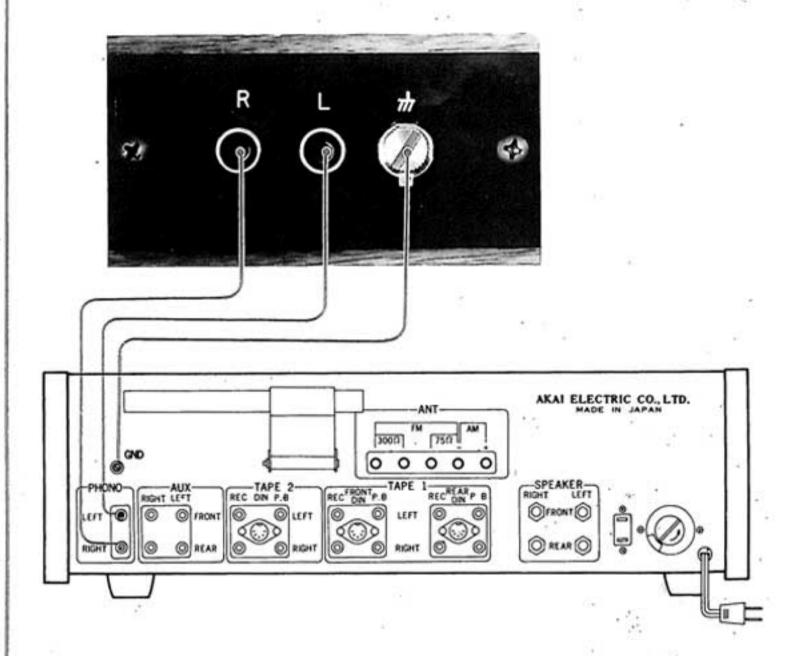
With standard accessory connection cord, connect the left (white) plug into the left output and the right (red) plug into the right output jack at rear of the AP-005, and connect the ground line to the # (ground) connection. Connect the other end of the cord to the external amplifier phono inputs, matching left and right, and connect the ground wire to the ground terminal of the amplifier.
